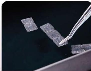
Black water tray and LED illumination to easily identify floating sections.
