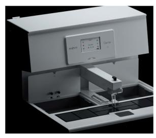
Modular embedding system with a 6L paraffin tank, a wide heated surface plus a wide cold plate, illuminated by LED working light. It has an easy to use display and user interface and comes equipped with an Ultrasonic sensor for wax dispensing.
