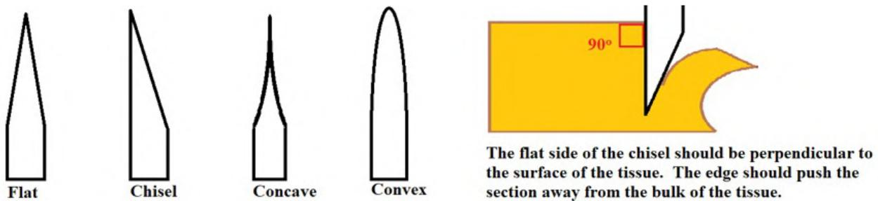
*Right: Four basic cross sections of a blade. Left: Using a chisel edge properly.*
